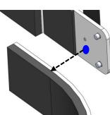
The screws must be tightened according to the above diagram. The notch marked with a blue point on part 4 corresponds to the hole indicated by the blue point mark on part 5.
