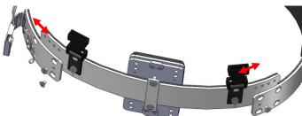
Finer adjustments of 6 mm can also be made by shifting the back plate of the lateral closing (10) (refer to the drawing below
